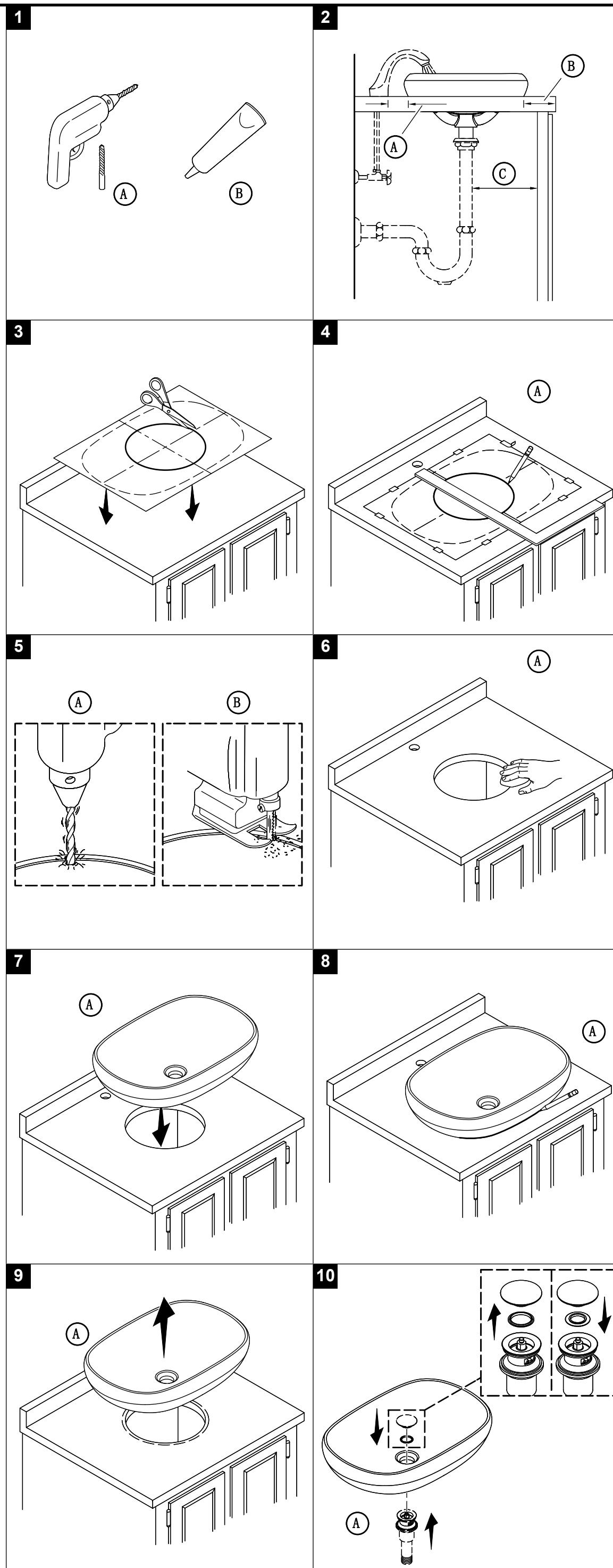
**10A.** Remove the drain cover and washer. Install the provided ceramic cover and the washer. Install the drain.
